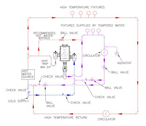
NOTE: Flow rates will vary depending on existing field conditions. Leonard Valve Company always recommends using CASPAK® sizing software for proper valve sizing and model number applications.
